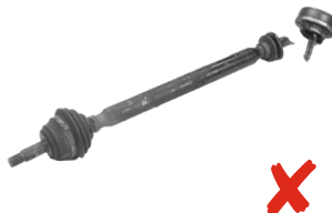
The shaft is incomplete – a joint has broken off.
