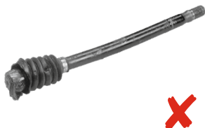
The shaft is incomplete – a joint is missing.
