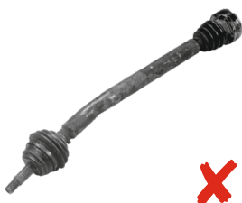
The shaft is complete but the profile shaft is bent.
