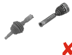
The profile shaft is broken.
